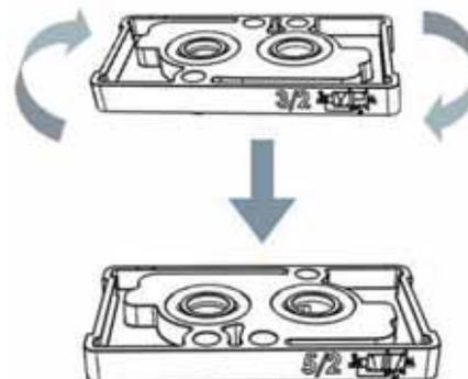
The V-Solenoid II™ rotary sealing plate results in less inventory
